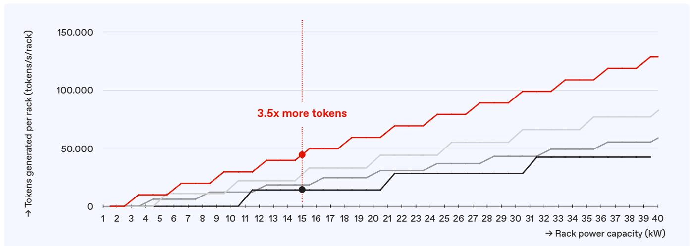
Comparison of rack-level token generation performance under a fixed 15 kW power budget, with all systems running identical workloads
